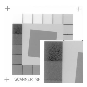
Figure 1. ISO Chart with artifacts due to the matt surface (brightened for better visualisation).
